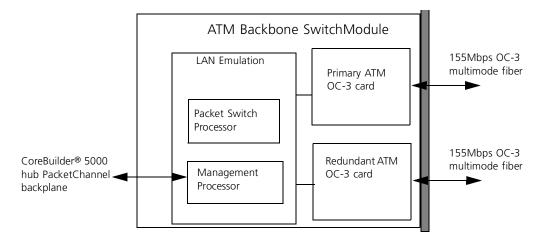
Figure 1-1 ATM Backbone SwitchModule Hardware Components
